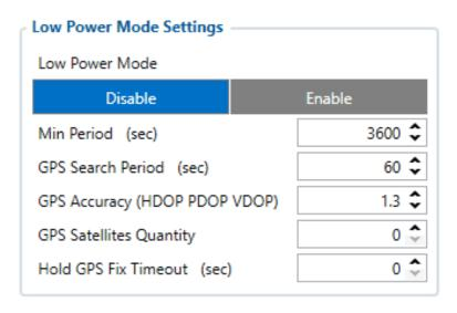
Low Power mode functionality was implemented to firmware from FMB.03.28.02.Rev.00. This functionality only works on devices that supports battery. It can only be active if device sleep mode
