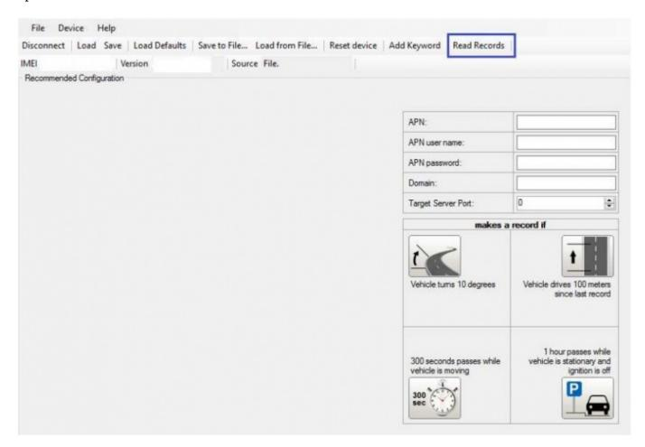
After device is switched on, you have to wait 3 minutes for device to startup. Only then it is possible to download records. If the memory is fully filled, the records reading may take several minutes. After reading records, all records are deleted from the device memory. Data records are stored in a binary file on your PC. You can upload these records from file to TAVL server and access all the data from TAVL. TAVL client application lets user to use the following features:
