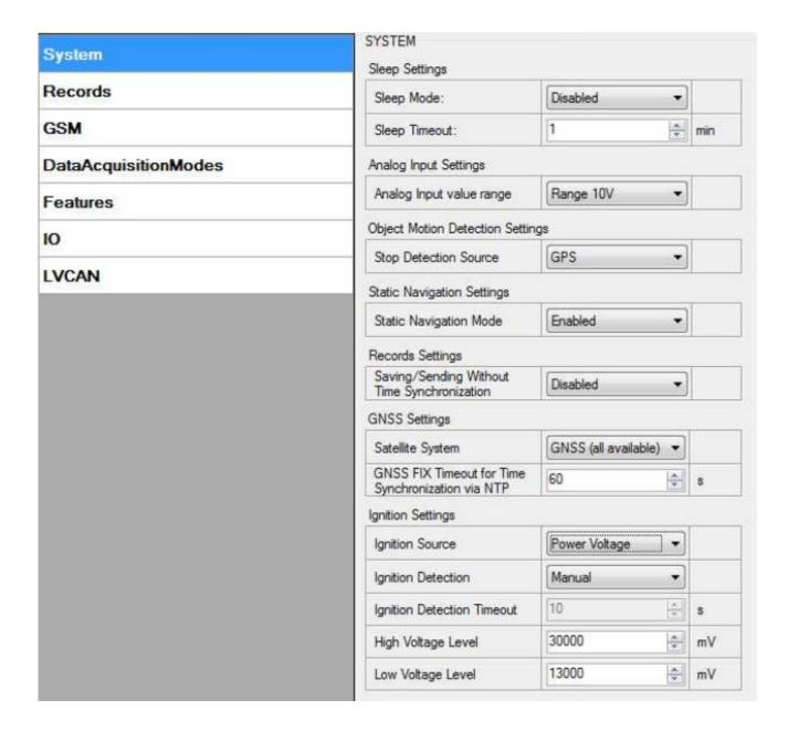
Also if Power Voltage is chosen for ignition source there is possibility to choose Manual ignition detection or automatic ignition detection. For manual ignition user has to choose power voltage levels by himself. For automatic ignition FM36M1 automatically detects ignition. In 12 V systems ignition is on when voltage is between 13,2 – 16 V and for 24 V systems ignition is detected when voltage is between 27 – 32 V.
