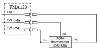
TTJ sensor pinout
