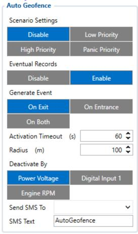
AutoGeofence is based on the last known position after the movement has stopped. You can be notified using this function if your car is taken away. The shape and size of Geofence zones are set by parameters. It is possible to state whether entering or leaving the geofence triggers an asynchronous message. AutoGeofencing options can be configured by following parameters as depicted in the right hand side figure:
