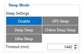
When in GPS sleep mode, FMB001 turns the GPS module off and continues making new periodic records. As a result power usage decreases, in turn saving vehicle battery.
