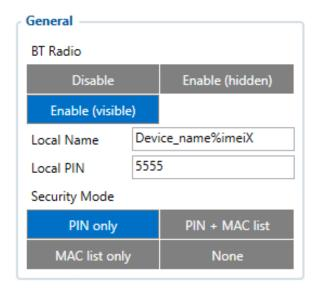
General functionality configures Bluetooth® to work in slave mode. This mode allows any external device to connect to FMB002.
