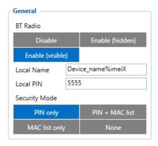
General functionality configures Bluetooth to work in slave mode. This mode allows any external device to connect to FMB020.
