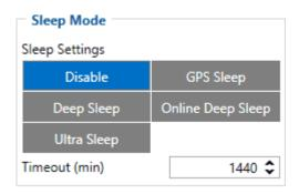
When in GPS sleep mode, FMB110 turns the GPS module off and continues making new periodic records. As a result power usage decreases, in turn saving vehicle battery.
