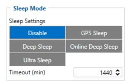
When in GPS sleep mode, FMB120 turns the GPS module off and continues making new periodic records. As a result power usage decreases, in turn saving vehicle battery.
