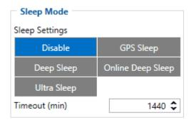
When in GPS sleep mode, FMB202 turns the GPS module off and continues making new periodic records. As a result power usage decreases, in turn saving vehicle battery.
