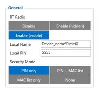
General functionality configures Bluetooth to work in slave mode. This mode allows any external device to connect to FMB204.
