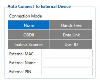
Auto connection functionality configures FMB204 as master device, which allows connecting FMB204 to an external device. FMB204 currently supports these modes:
