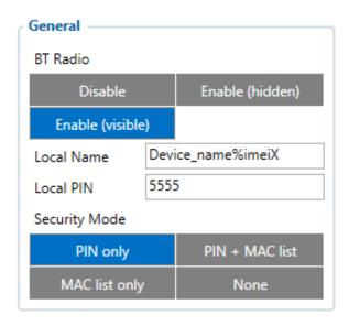
General functionality configures Bluetooth to work in slave mode. This mode allows any external device to connect to FMB209.
