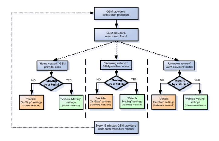
The operator search is performed every 15 minutes. Depending on the current GSM operator Home, Roaming or Unknown mode can be changed faster than every 15 minutes. This process is separate from the operator search. Movement criteria are checked every second.
