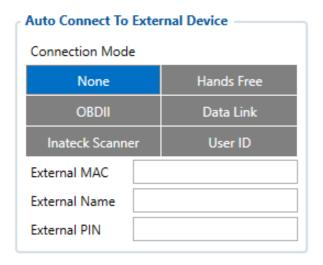
Auto connection functionality configures FMB225 as master device, which allows connecting
