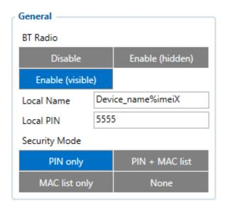
General functionality configures Bluetooth to work in slave mode. This mode allows any external device to connect to FMB225.
