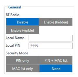
General functionality configures Bluetooth @ to work in slave mode. This mode allows any external device to connect to FMB230.
