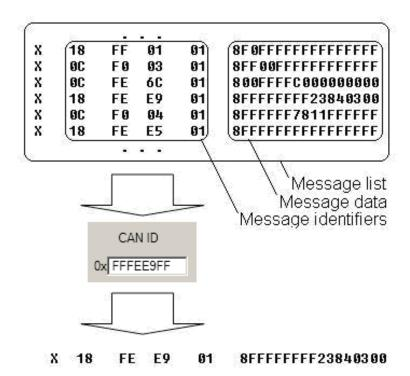
When certain message is filtered, FMB630 checks which data bytes should be sent to server. Document indicates that 5-8 bytes are used in FMS standard.
