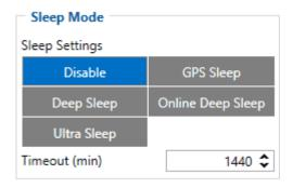
When in GPS sleep mode, FMB630 turns the GPS module off and continues making new periodic records. As a result power usage decreases, in turn saving vehicle battery.
