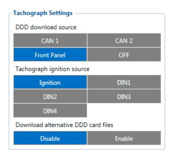
It allows to download DDD file data from tachograph front interface K-Line (Pin2 in front connector). To configure the device simply select "Front Panel" to be DDD download source.
