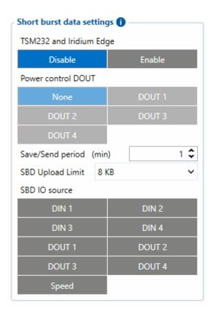
**Save/Send period** configures how long will FMB device wait after losing the signal to generate SBD packet. If the signal is not recovered, it will send it indefinitely (or till the SBD Upload limit is reached, if such is set).
