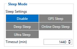
Please note that power saving depends on two configurable parameters: *Send Period* and *Minimum Record Saving Period* in "X on Stop Mode". When records are sent successfully in deep sleep mode, open link timeout counter will be skipped and FMB910 Basic will enter deep sleep mode immediately.
