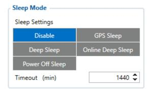
When in GPS sleep mode, FMB965 turns the GPS module off and continues making new periodic records. As a result power usage decreases, in turn saving vehicle battery.
