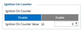
**Ignition ON Counter** scenario counts the time spent with the ignition in the resolution of seconds. It is possible to configure a starting value of the counter. Maximum value: **2147483647** seconds or 596523.235 hours **NOTE THAT**, when entering a starting value, the value must be in seconds!
