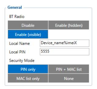
General functionality configures Bluetooth to work in slave mode. This mode allows any external device to connect to FMC00A.
