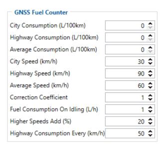
To configure *Fuel Counter* parameters use fuel consumption norms which are presented in the technical documentation of the vehicle. By default speeds for these fuel consumption norms are: City – 30 km/h, Average - 60 km/h, Highway - 90 km/h. These values can be changed.
