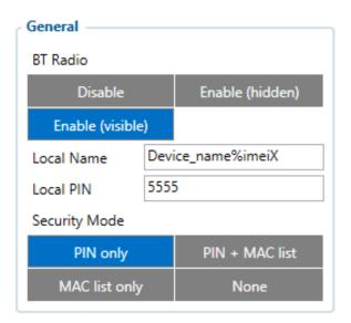
General functionality configures Bluetooth ${}^\circledR$  to work in slave mode. This mode allows any external device to connect to FMC150.
