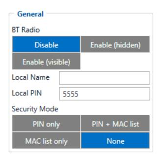
General functionality configures Bluetooth to work in slave mode. This mode allows any external device to connect to FMC225.
