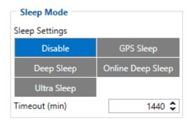
When in GPS sleep mode, FMC150 turns the GPS module off and continues making new periodic records. As a result power usage decreases, in turn saving vehicle battery.
