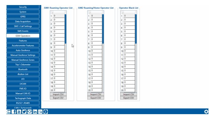
If roaming operator list is left empty, FMC640 will automatically detect home operator. If home operator is written to the roaming operator list, it will still be detected as home operator. Any operator not in the roaming operator list (except the home operator) will be recognized as unknown operator and FMC640 will work in Unknown mode (make sure it is configured to allow data sending – GPRS context is enabled).
