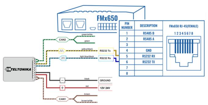
LV-CAN200 connection example. This is not a connection diagram for your vehicle. Every vehicle has a specific scheme.
