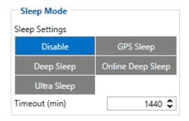
When in GPS sleep mode, FMC650 turns the GPS module off and continues making new periodic records. As a result power usage decreases, in turn saving vehicle battery.
