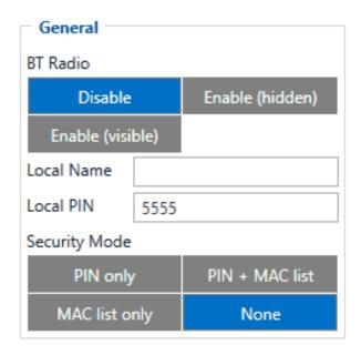
General functionality configures Bluetooth to work in slave mode. This mode allows any external device to connect to FMM125.
