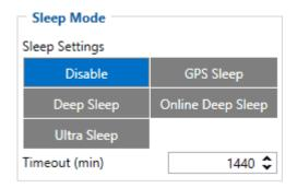
When in GPS sleep mode, FMM130 turns the GPS module off and continues making new periodic records. As a result power usage decreases, in turn saving vehicle battery.
