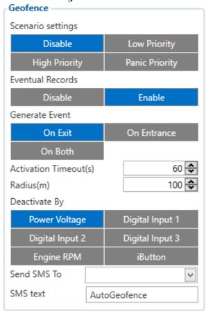
*AutoGeofence* is based on the last known position after the movement has stopped. You can be notified using this function if your car is taken away. The shape and size of Geofence zones are set by parameters. It is possible to state whether entering or leaving the geofence triggers an asynchronous message. AutoGeofencing options can be configured by following parameters as depicted in the right hand side figure:
