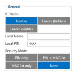
General functionality configures Bluetooth to work in slave mode. This mode allows any external device to connect to FMM230.
