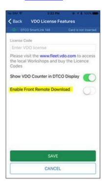
To check if your tachograph is already enabled (**by default**, from the factory, remote DDD files from Front Interface is **disabled**) you can contact your VDO service or use "tachocheck" SMS command.
