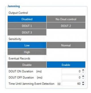
When jamming is detected the scenario is activated, an event record is generated and digital output status is changed to 1 when configured once *Jamming* timeout runs out. If jamming ends during timeout countdown no event will be generated and output will not be controlled. *Eventual Records* parameter can be configured: when it is disabled scenario status value will appear in each AVL record, otherwise it will be appended only to eventual records.
