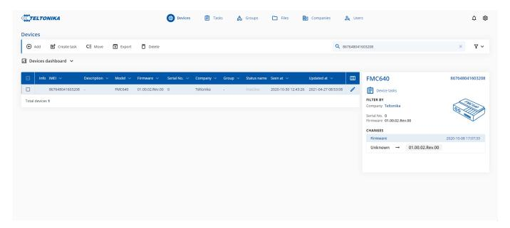
Once the firmware update task has been assigned, it can be seen in the main window. Please note that uploading will start after the next scheduled connection to Fota Web. The instant connection to the FOTA WEB can be initiated by an SMS command "web\_connect".
