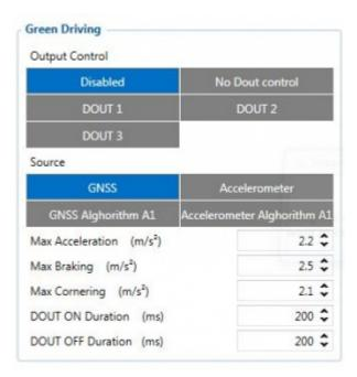
When vehicle parameters exceed the values of *Max Acceleration, Max Braking* or *Max Cornering* parameters, the scenario is activated: a record is generated and digital output status is changed to 1 when configured. You can configure all three parameters in m/s² units. Scenario is activated until current Acceleration, Braking or Cornering value decreases below the set parameter value. Parameters used with *Green Driving* functionality are given in a table below.
