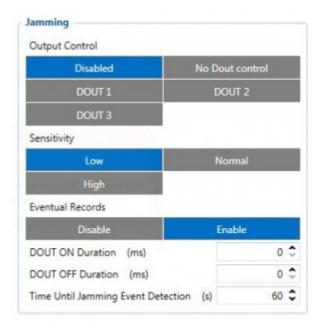
When jamming is detected the scenario is activated, an event record is generated and digital output status is changed to 1 when configured once *Jamming* timeout runs out. If jamming ends during timeout countdown no event will be generated and output will not be controlled. *Eventual Records* parameter can be configured: when it is disabled scenario status value will appear in each AVL record, otherwise it will be appended only to eventual records.
