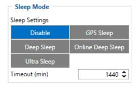
When in GPS sleep mode, FMM80A turns the GPS module off and continues making new periodic records. As a result power usage decreases, in turn saving vehicle battery.
