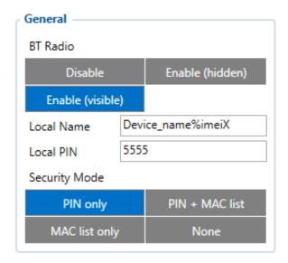
General functionality configures Bluetooth® to work in slave mode. This mode allows any external device to connect to FMM880.
