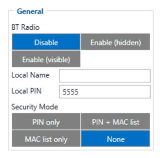
General functionality configures Bluetooth® to work in slave mode. This mode allows any external device to connect to FMP100.
