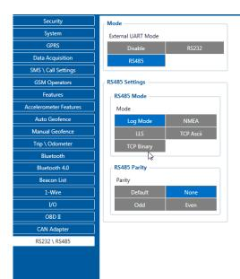
TCP Binary has a setting Prefix. It is possible to set Prefix 1, Prefix 2 or Prefix 3. These prefixes can be used seperately or in unison. To configure this setting a value from 0 to 255 in decimal has to be entered. Device will convert this value to HEX and compare the 1st, 2nd or 3rd byte from incoming data. If the values do not match, device will not accept incoming data.
