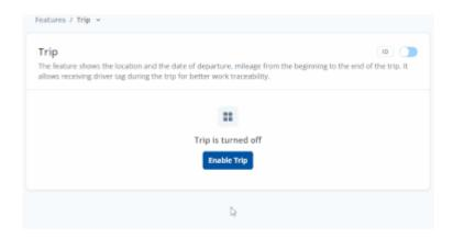
*Trip* section offers user to configure the *Trip* feature. *Trip* starts when Ignition according *Ignition* source is ON and Movement according *Movement source* is ON and also 'Start Speed' is exceeded. *Start Speed* defines the minimum GPS speed in order to detect *Trip* start.
