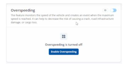
When the vehicle speed exceeds the configured maximum speed value, the scenario is activated, and an event record is generated and digital output status is changed to 1 when configured. Detected speed has to be greater than configured max speed +3% of configured max speed for the overspeeding event to start. To stop the overspeeding event, the detected speed has to be lower than the configured max speed -3% of the configured max speed. Configurable parameters:
