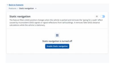
Static Navigation Mode is a filter, which filters out track jumps when the object is stationary.
