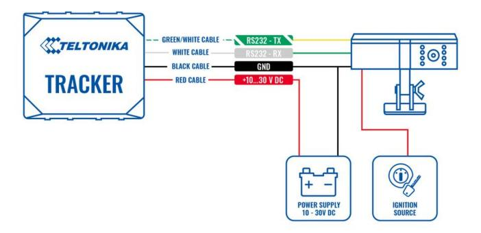
If you need to receive additional data from the DualCam when the ignition is off, you can do it by connecting the camera to a power source using the relay, to control the power supply by turning on/off the camera. To find information on how to configure DOUT, please visit <u>FMB DOUT</u>.
