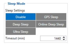
When in GPS sleep mode, GH5200 turns the GPS module off and continues making new periodic records. As a result power usage decreases, in turn saving vehicle battery.
