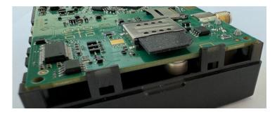
Devices ordered with client SIM cards will have both the 'dummy' SIM card in the top (SIM2) slot and the client SIM card in the
