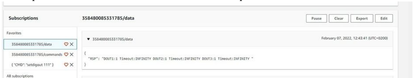
Figure 32. Response to a command in the data topic, the command was published in command topic
