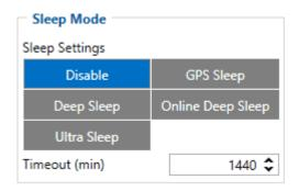
When in GPS sleep mode, MTB100 turns the GPS module off and continues making new periodic records. As a result power usage decreases, in turn saving vehicle battery.
