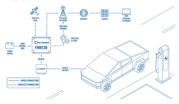
When installing FMB130 in a vehicle, follow the **mounting recommendations.** When connecting to the **CAN bus**, you must use the diagrams provided by our technical support engineers. The diagrams indicate in detail and clearly the connection points in the vehicle wiring and the required program number.
